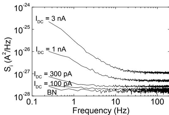
Fig. 4. Power spectral density of the current noise measured in a 7 nm thick oxide MOS structure at different DC current levels. The background noise (BN) of the transresistance amplifier is also shown.
